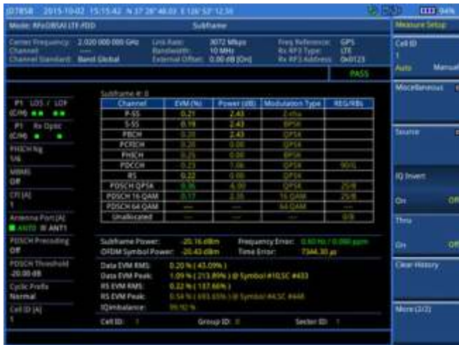
RFoBSAI LTE-FDD signal analyzer window
