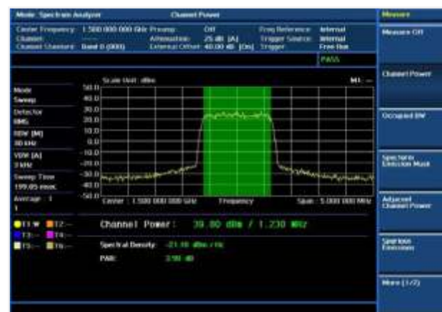
RF test Channel Power
