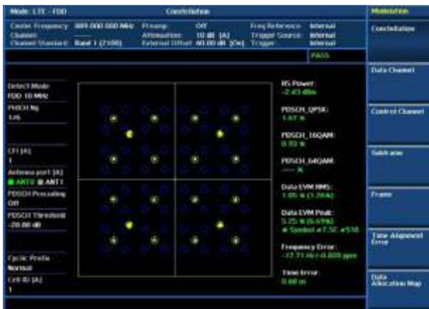
Modulation analysis — Data Constellation
