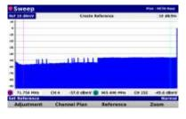
test and set the tilt and gain of distribution amplifiers without the need for any dedicated headend gear
