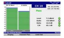
Carrier-to-Noise measurements when compared against user-defined limit sets
