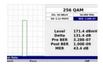
This feature doesn't require any expensive headend sweep gear and works with any DOCSIS 3.0 or DOCSIS 3.1 compatible CMTS with pre-EQ enabled
