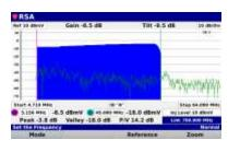
suck-outs between the test point and the headend, while also stepping around active channels in order to avoid interference
