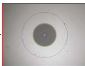
Fail: particle inside zone A
