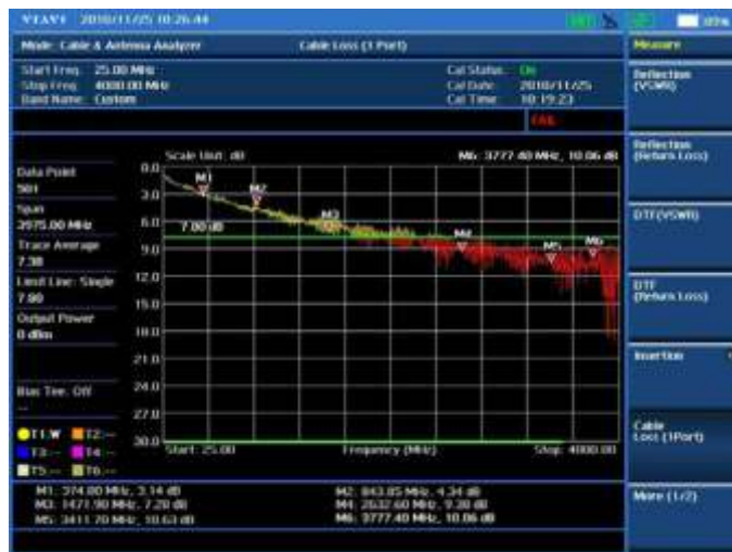
Cable and antenna test — Cable Loss
