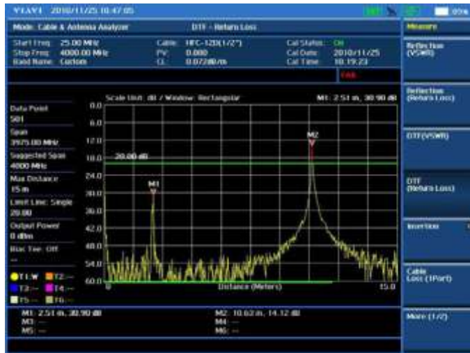
Cable and antenna test — Distance to Fault
