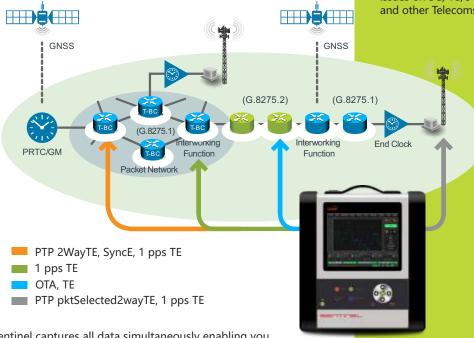
Sentinel captures all data simultaneously enabling you to correlate timing performance at different points in the network, even between different timing architectures.
