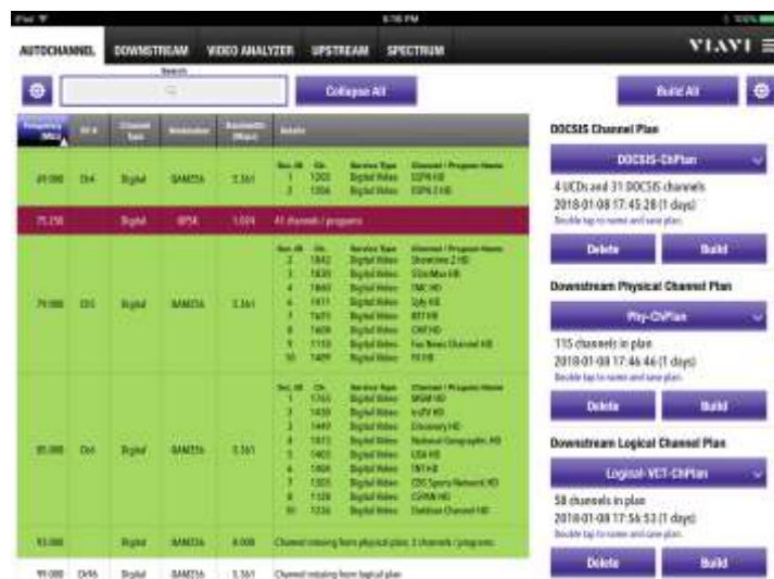
The VSE-1100 allows the user to build, save, delete, and rename multiple channel plans.
