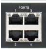
The four GbE ports provide network configuration flexibility and enhanced security. Multiple isolated and synchronized time servers can also be configured. Two 10 GbE SFP+ ports can be added for NTP/PTP operations as well.
